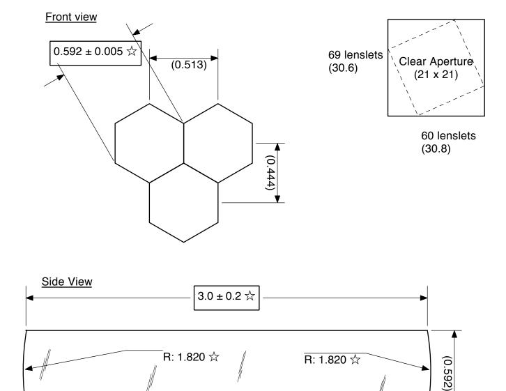
SED Machine Lenslet Array (run 57r, rotated 20.919 degree) Nick Konidaris (npk@caltech.edu) +1 831 704 6425 2 Jan 2012 For reference: Surface Sag 24  $\mu$ Focal length: 2.66
